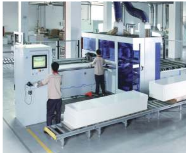
▼ German Homag Drilling Machine Computer Controlled
